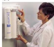
As long as the green LED is on, the water quality is above 1 MΩ·cm at 25°C. When the LED is red, it's time to change the purification pack (DI-PAK)™.
